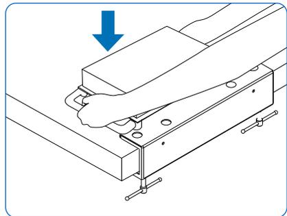
The build platform jig is designed to stabilize the build platform for the secure removal of prints. Secure the build platform jig to the edge of your work surface by tightening the jig screw clamps underneath the work surface. The build platform jig can also be secured to the work surface using the two screw holes on the front of the jig. Ensure that there is enough space in front of the jig for the build platform.
