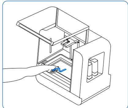
6. Rest the long edge of the tank tool on the flexible film interior. Skim the film surface. Search for obstructions that indicate cured resin stuck to the flexible film.
