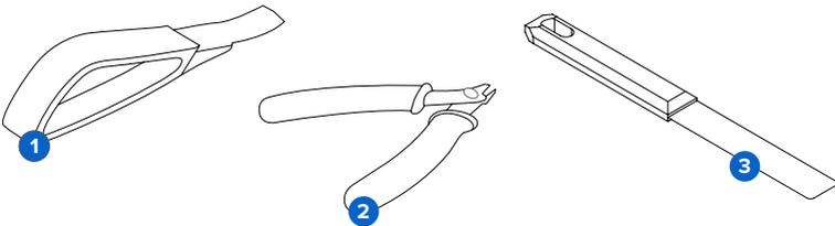
The accessories include sharp tools such as: a removal tool **1**, flush cutters **2**, and a scraper **3**.
